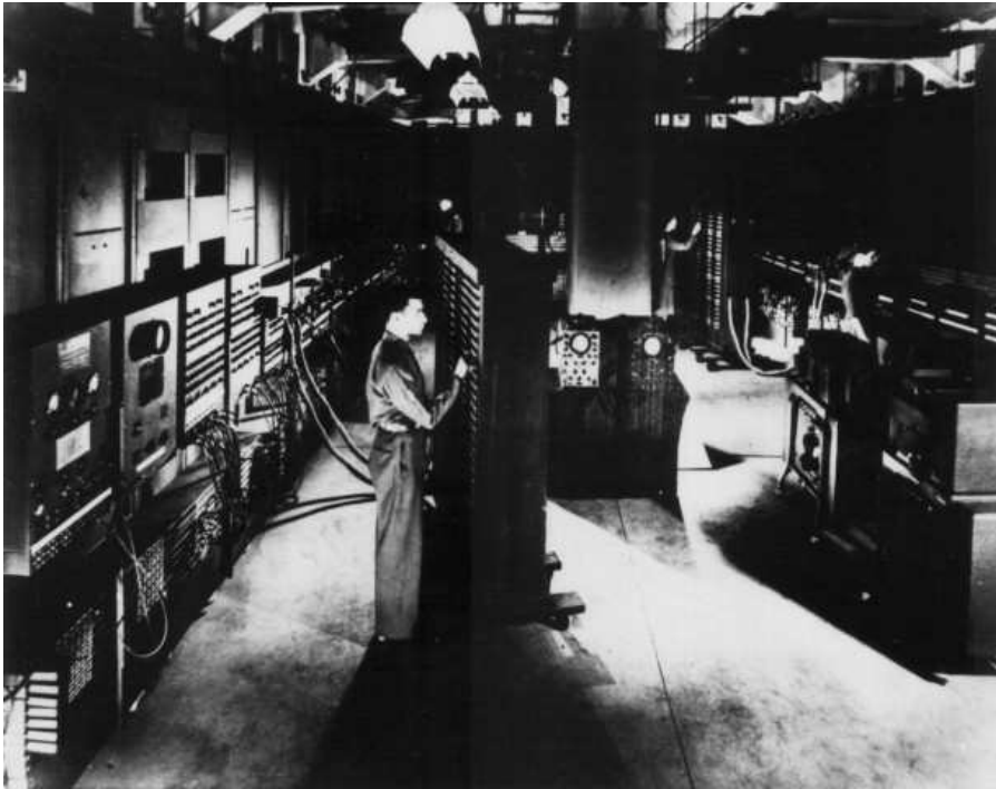
Irwin Goldstein (foreground) sets the switches on one of the ENIAC's function tables at the Moore School of Electrical Engineering
